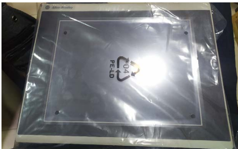
Figura 60. HMI Panel View 800 de Allen Bradley
